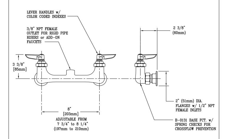
NOTE: RIGID BASE MAY BE CONVERTED TO SWIVEL BY SPECIFYING B-0412 RIGID to SWIVEL ADAPTER.
