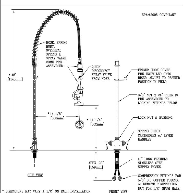
Product Description: Drawn: Checked Scale: EASY INSTALL PRE-RINSE UNIT: RJK JRM 1:8 SINGLE DECK MOUNT BASE MIXING FAUCET, FLEXIBLE SUPPLY HOSES, 24" RISER, Date: Approved SUPPORT SPRING, 44" FLEX HOSE w/ QUICK DISCONNECT, B-0107 SPRAY VALVE 01/04/06 JHB
