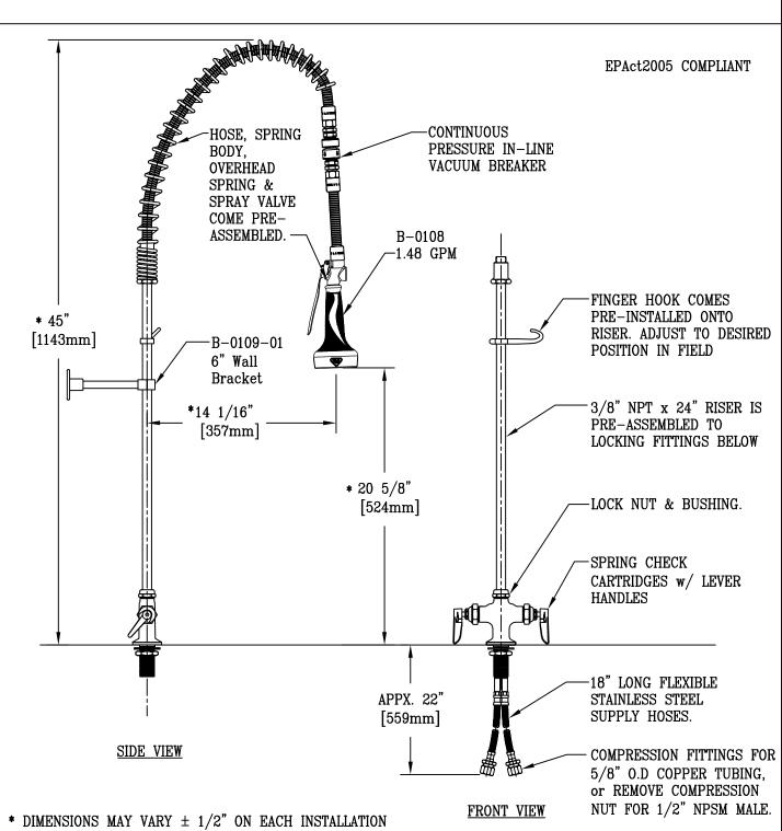
Product Description: Drawn: Checked Scale: EASY INSTALL PRE-RINSE UNIT: JRM **WJS** 1:8 SINGLE DECK MOUNT BASE MIXING FAUCET, FLEXIBLE SUPPLY HOSES, 24" RISER, Date: Approved SPRING, 44" FLEX HOSE w/ VACUUM BREAKER, B-0108 SPRAY VALVE, WALL BRACKET 08/09/06 JHB
