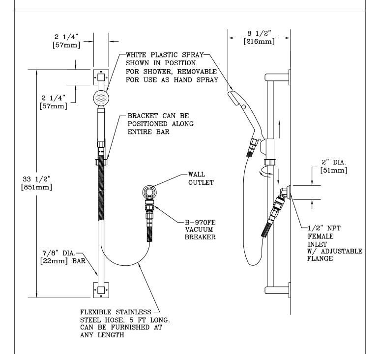
NOTE: SIX MOUNTING SCREWS FURNISHED WITH EACH BAR, WHEN SECURELY MOUNTED ON WALL, BAR SERVES AS GRAB BAR.
