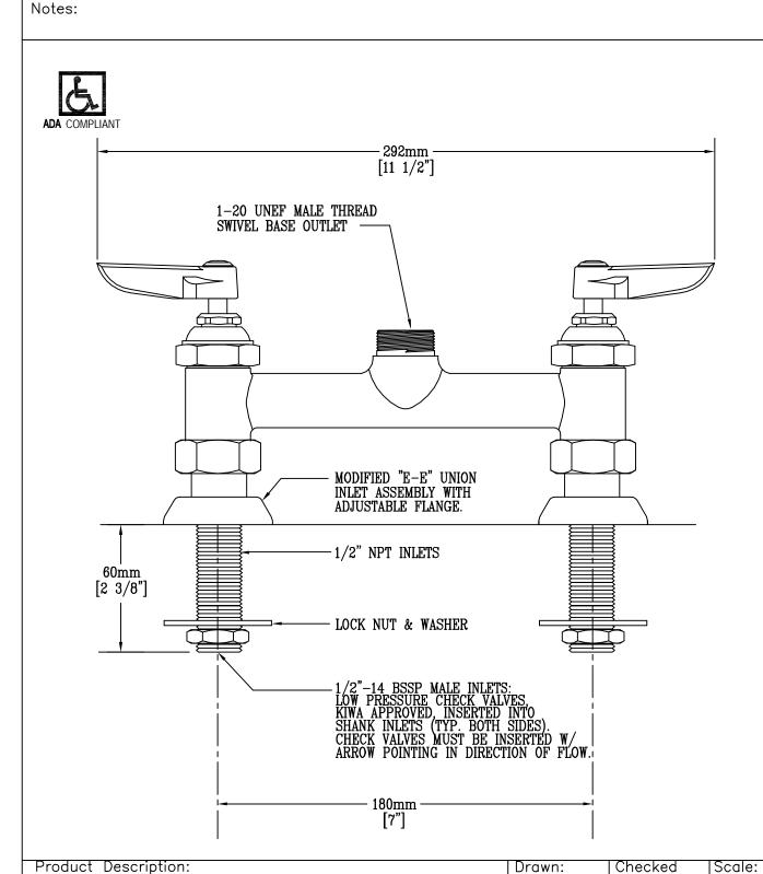
180mm SWIVEL BASE FAUCET WITH MODIFIED "E-E" INLETS, LEVER HANDLES, & 1/2" BSSP MALE INLET SHANKS
