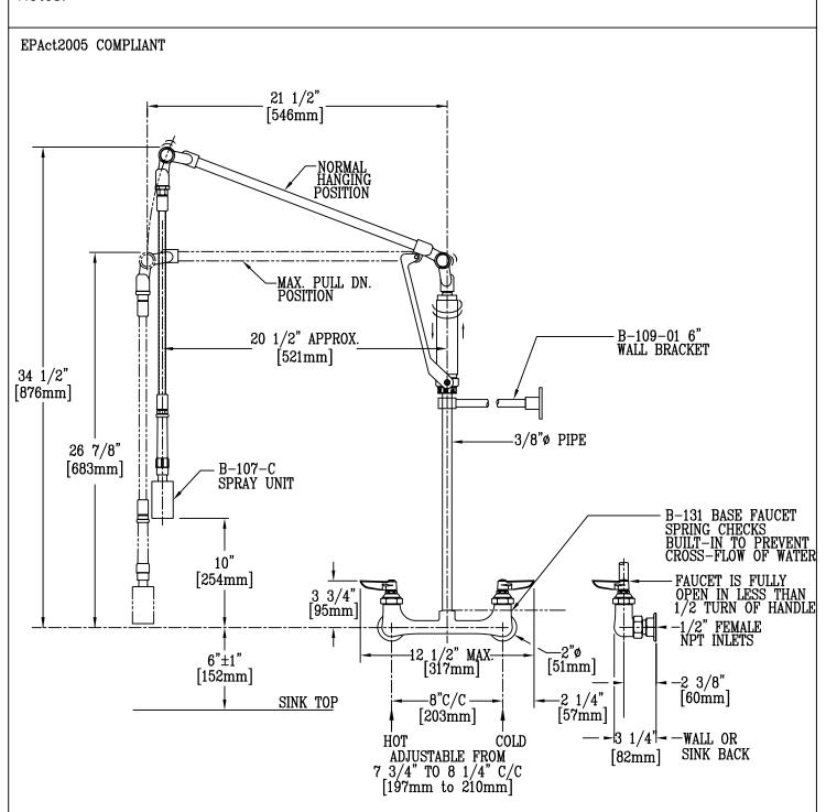
NOTE: FOR BACKSPLASH MOUNTING, RISER MUST BE SHORTENED TO MAINTAIN 10 3/4" [273mm] CLEARANCE BETWEEN SPRAY HEAD AND FIXTURE FLOOD RIM LEVEL.
