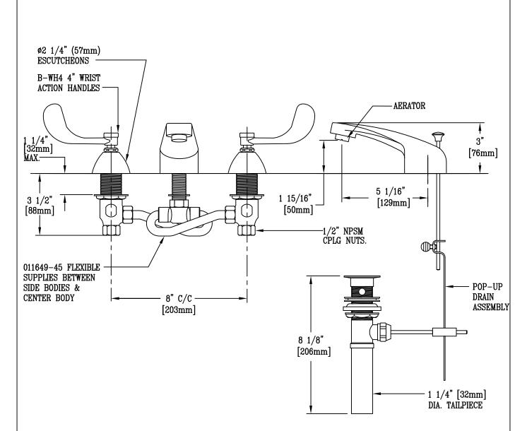
NOTE: ROUGH-IN REQUIRED: \$\phi7/8\$ FOR CENTER SHANK \$\phi1 1/4\$ FOR HOT/COLD SIDE BODIES
