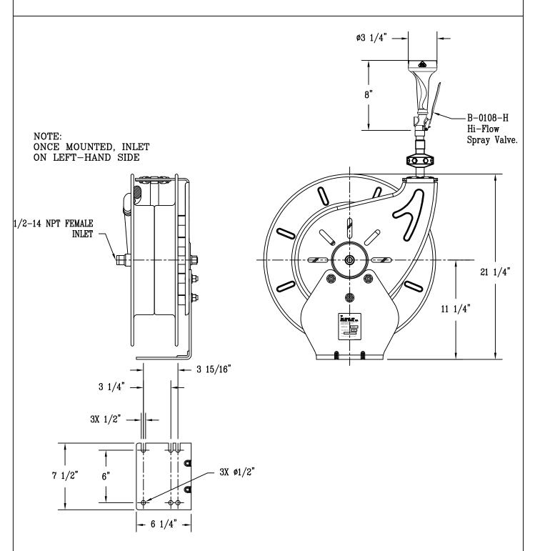
Hose Reel: Open, Epoxy Powder Coated Steel, 35 FT of 1/2" Dia. Blue Hose and
