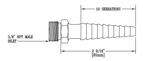
NOTE: BL-5550-25 SERRATED TIP IS USED ON SIDE OUTLETS OF TURRETS, OUTLETS, OR PANEL FLANGES, AND IN OTHER APPLICATIONS IN WHICH A SMALL HEX SHOULDER IS NECESSARY TO AVOID INTERFERENCE OR CONTRIBUTE TO APPEARANCE.
