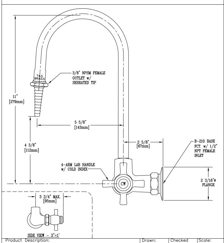
LABORATORY SINGLE SINK FAUCET WITH RIGID GOOSENECK, 4—ARM HANDLE, SERRATED TIP, 1/2" NPT FEMALE INLET
